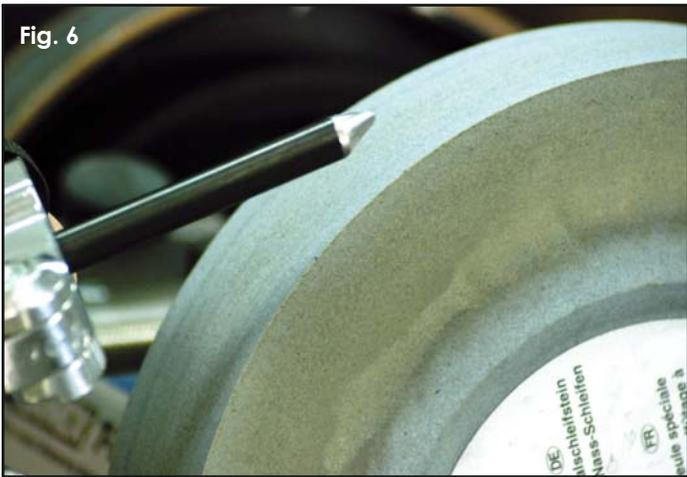
The real test, I thought, would come when I moved to the water-cooled wheel to see how accurately the dry ground tool would mate with the wheel on the T-7. As shown in **Fig. 5**, it was perfect. It took only seconds to refine the surface finish and the bevel. You can see the end result in **Fig. 6**.
