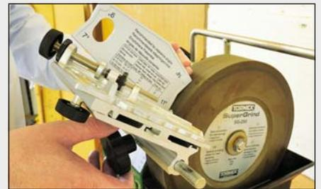
Tilt the base up and set it to the required clearance angle using the template
