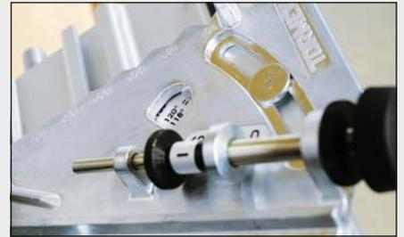
Set the point angle on the guide before sliding it onto the base plate
