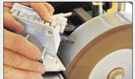
I found it best to give the nut 1½ turns, grind both sides and gradually adjust the stop nut to sneak up on the primary facet
