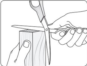
Do not hone the edge after grinding! There is no need for a finer surface. As a matter of fact a coarser surface on the scissors makes them work better, as the material (cloth or paper) to be cut slides less and cuts more easily. Remove the little burr resulting from the grinding by drawing the scissors through the end grain of a piece of wood.
