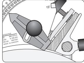
If you want to grind a new edge angle, use the AngleMaster WM-200. Let the indicator touch the holder between the two clamps.
