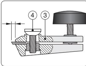
Adjust the screw (4) so the clamp (3) fits the scissor thickness. Leave about 3 mm ( $\frac{1}{8}$ " ) protruding.
