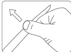
Grind until you have a burr along the entire length of the blade, and you can see an evenly ground bevel.
