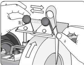
Grind carefully by placing the jig on the support plate with a light downward pressure.
