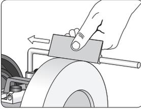
Slide the support plate onto the Universal Support. Lock the Universal Support in the lowest possible position with clearance for the plate.
