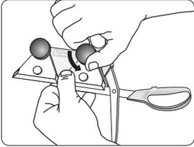
Remove the partially ground scissors from the jig by loosening the large knob.
