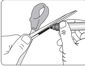
If you want to repeat the existing edge angle, colour the bevel with a marker to see where the grinding will take place.
