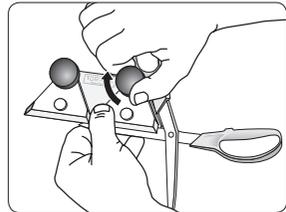
Ensure that the other blade will remain clear of the side of the wheel and tighten the large knob to hold the scissors in place.
