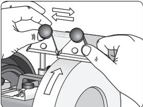
These are ground the same way as scissors. The bevel and back should however be honed. After grinding, keep the blade in the holder and hone the bevel and the back alternately until the burr disappears.
