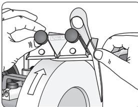
Move the jig back and forth across the wheel while following the shape of the blade.
