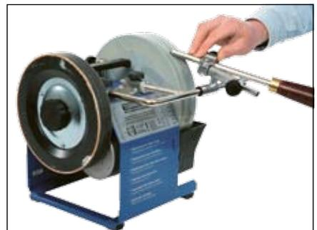
Slide the jig and roll the tool from side to side
