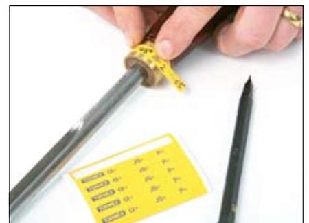
The pen and set of labels (included) mean you can label each tool with its sharpening 'recipe'
