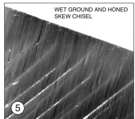
Photo 5. In this case the **wet grinding** method has been used in conjunction with the honing wheel. Note the clean polished edge.
