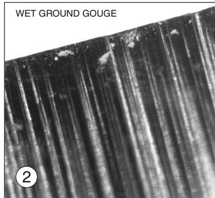
Photo 2. A gouge ground using the **wet-grinding** method, with the direction of rotation away from the tool edge. The view is into the flute of the gouge.
