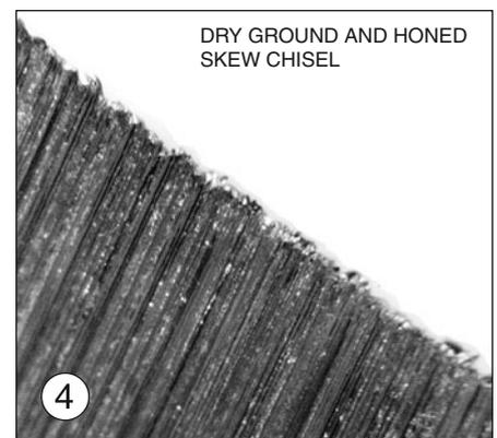
Photo 4 is after honing. Note the duller look of the honed surface and the root of the burr firmly in place.
