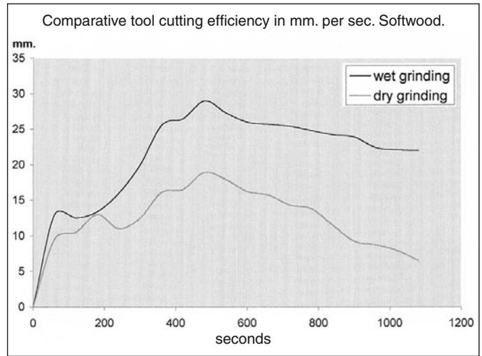
This graph shows the results of trials performed with softwood A standard, group one joinery quality pine was used, and selected to be reasonably knot free. Both tools can be seen to maintain their edge for a longer period, but the trend for the wet-ground tool to achieve higher results is maintained. Notice the point at which the dry-ground burr disappears. Also of note is the fact that both tools mirror some upward performance trends, caused by timber density, etc.
