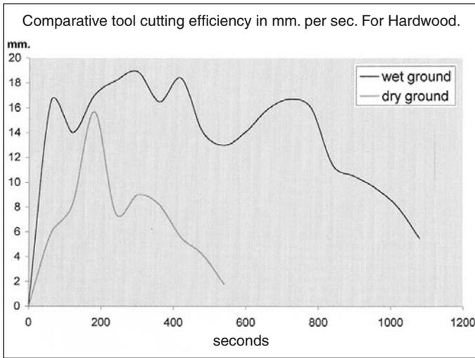
This graph shows the collective results of both tool grinding methods for hardwood. The path lines on all the graphs are seen to undulate. This is because the data has been reproduced without any statistical manipulation. This graph, shows very clearly, the peak at which the burr was worn away from the dry-ground tool.
