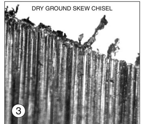
Photos 3 & 4. Show an attempt at burr removal on a skew chisel. In photo 3 the burr has been produced by the **dry-grinding** method straight from the wheel.
