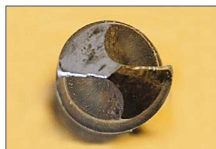
This close-up shows a standard twist drill bit in need of sharpening
