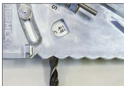
Check the bit's point angle by holding it against a groove on the edge of the guide
