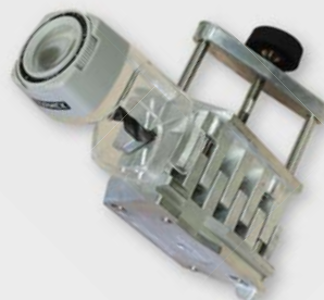
Turn the drill bit to align its cutting edge with the lines on the holder; use the magnifier if needed
