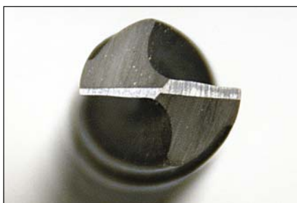
This image reveals the four-faceted point of a freshly-sharpened bit
