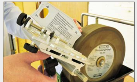
Tilt the base up and set it to the required clearance angle using the template
