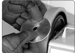
**⚠** Use protective gloves to help prevent cuts! Ensure that the honing wheel rotates **from** the edge, otherwise the blade will cut into the honing wheel.
