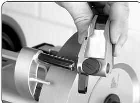
Remove the knife jig from the machine and replace it with the RBS-140 Round Blade Sharpening Attachment (hereafter referred to as the "Accessory").
