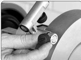
Remove the supplied stop ring and attach it to the machine's shaft against the Accessory to hold it in place.
