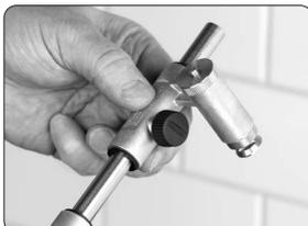
To set the size, loosen the guide's stop screw and slide it to the desired size. Tighten the stop screw again to lock.
