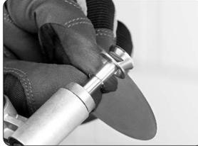
Thread the tensioner through the blade hole with the bevel against the thick end. Refit the tensioner and the blade in the guide.
