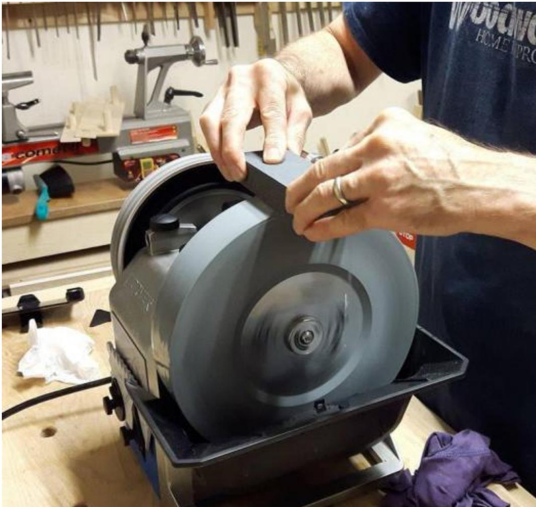
*The grindstone being 'converted' from 220 to 1000-grit*
